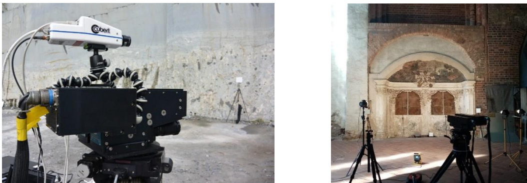
Figure 26 HySpex Sensors and Cubert Camera mounted on rotation stage to scan a cultural site in close-range (Marienkirche, Frankfurt Oder, Germany).
